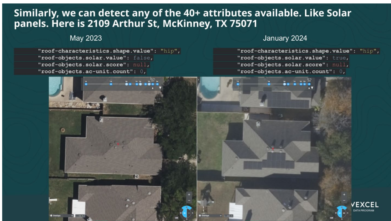
Figure 14: Detection of Specified Attributes. Using machine learning, models can detect the presence of solar panels on a roof in Texas. The ability to detect certain features will enhance valuation accuracy.
