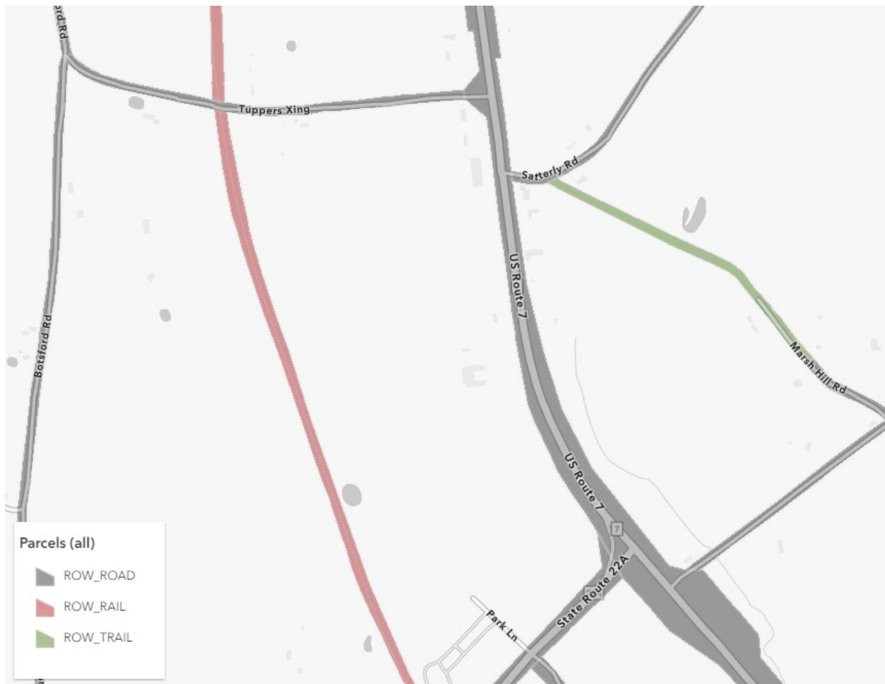
Figure 9: Rights-of-Way Types. Example of parcels with Property Type of ROW_Road (grey), ROW_Rail (red), and ROW_Trail (green) in Ferrisburgh.
